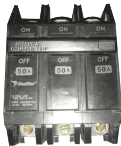
Breaker TQC1215W 3P 50A 120/240VAC 50/60Hz SeaStar
