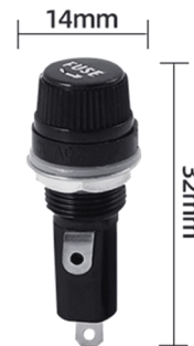
Portafusibles Americano 15A 125VAC, 10A 250VAC 6X30MM
